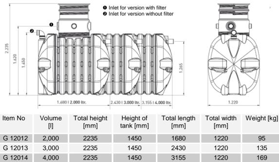
Tab: available tank sizes with integrated filter; all sizes also available without filter (different item No).
