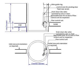
Flow control systems are essential to regulate storm water flow before discharging into water courses or sewer networks. Aquality Storm water Flow control chambers are designed as a totally integrated solution to this problem. Our chambers are fabricated through a range of depths and diameters to meet precise containment and flow criteria.
