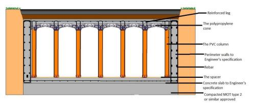
and cost effective way of achieving a strong concrete water storage void with a very high load bearing capacity and therefore suitability for heavily trafficked areas. The Aquality Goliath formwork makes it possible to create reinforced concrete tanks of custom depth by using the PVC columns supplied to the required length.
